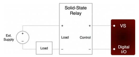
Figure 2.8.1.4-1. Relay Connections (Sinking Control, High-Side Load Switching)
