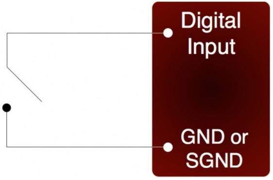
Figure 2.8.1.3-1. Basic Mechanical Switch Connection To Digital Input
